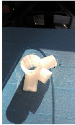
Fig.11. Obtained part through FDM (Fused deposition modeling)
